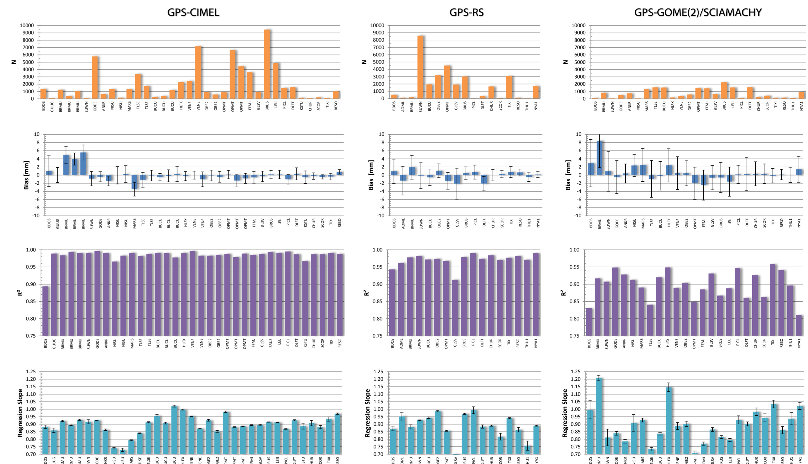
Fig. 4: Column bar plots of scatter plot properties (count N, bias, R^2 and regression slope) of the different instruments versus GNSS for the selected sites worldwide. Sites are ordered with increasing latitude. The error bars represent the RMS (bias) and the standard deviation (regression slope).
