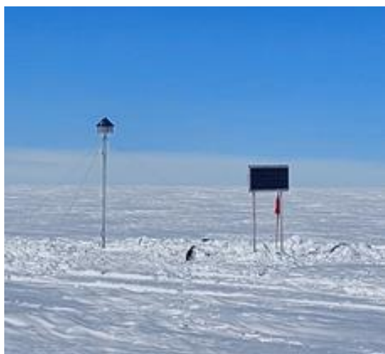
Left image: Autosampler for inorganic analyses of ULB with solar panel and curious penguin; right image: the passive and active sampling system for VOCs and partially oxidised VOCs of UGent on the roof of the southern science shelter at PES
