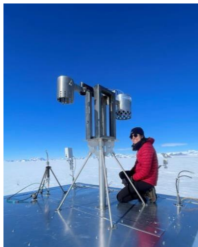
Left image: Autosampler for inorganic analyses of ULB with solar panel and curious penguin; right image: the passive and active sampling system for VOCs and partially oxidised VOCs of UGent on the roof of the southern science shelter at PES
