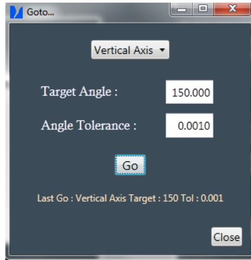
After selecting the Axis, Angle and Tolerance you can execute the goto command. AutoDIF moves in the desired position. The window stays open until the close button is pressed. This makes possible to execute a sequence of goto commands, typically needed during levelling of the instrument. The last executed goto command is shown in the label. Pressing the close button does not stop the movement (operator needs to press the reset button in the toolbar).
