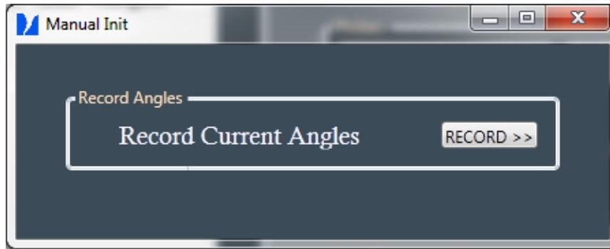
Press the save button to register the position and complete the manual initialization.
