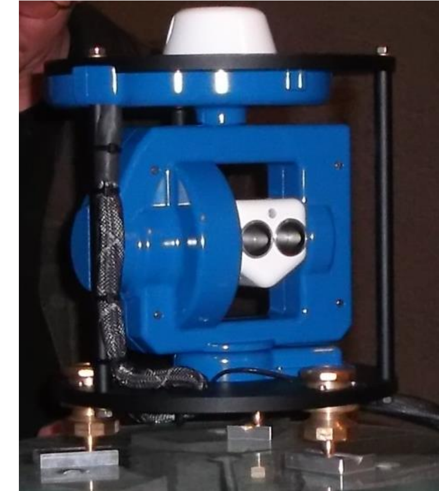
Right: the Autodif is an Automated Diflux for magnetic observatories (azimuth reference is provided by an embedded laser pointing a reflector). The Gyrodif instrument is an Automated Diflux for remote applications (an embedded gyroscope provides the azimuth reference)
